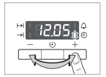
After approx. 5 seconds, the flashing stops and the clock displays the time set.
